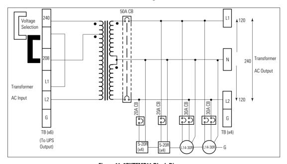
Figure 11. 9PXTFMR11 Block Diagram
