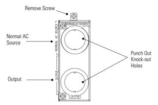
Figure 9. Removing the Terminal Block Cover
