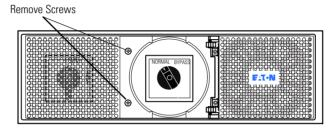
Figure 17. Remove the Front Cover Screws
