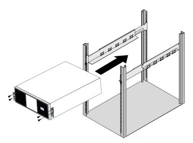
Figure 5. Installing the Cabinet in the Rack
