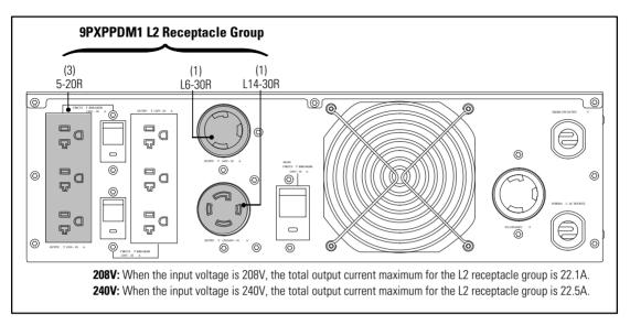
Figure 28. 9PXPPDM1 L2 Load Output Limits
