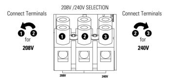
Figure 22. Wire Selected Voltage
