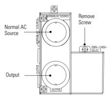
Figure 21. Remove the Voltage Selection Terminal Block Cover
