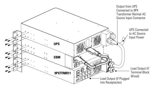
Figure 33. 9PXTFMR11 and 11k 240V EBM with 9PX11000 UPS (Kit 9PX11KTF11)
