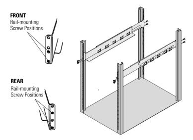
Figure 3. Attaching the Rails
