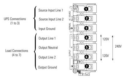
Figure 10. 9PXPPDM2 I/O Terminal Block
