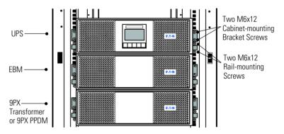
Figure 6. Cabinet installed in Rack (Front view)
