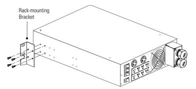
**Figure 4. Installing Mounting Brackets**
