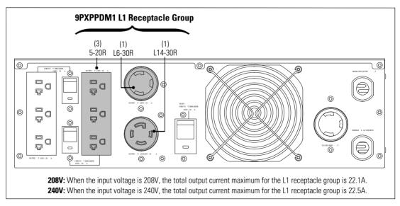
Figure 27. 9PXPPDM1 L1 Load Output Limits
