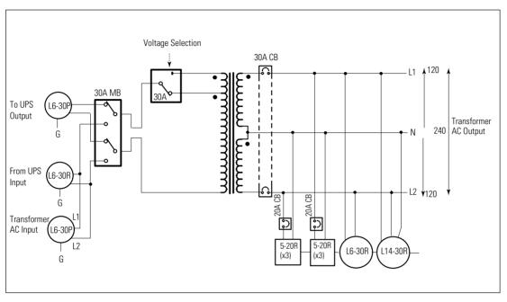
Figure 14 shows the 9PXPPDM1 block diagram.
