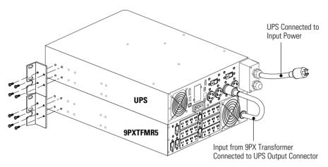
Figure 29. 9PXTFMR5 with 9PX5000 or 9PX6000 UPS (Kits 9PX5KTF5 and 9PX6KTF5)
