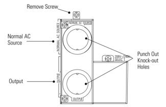
Figure 12. Removing the Terminal Block Cover
