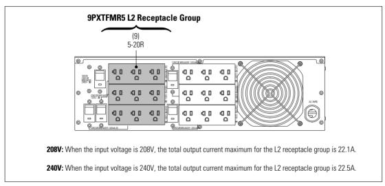
Figure 24. 9PXTFMR5 L2 Load Output Limits
