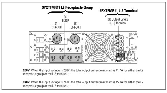
Figure 26. 9PXTFMR11 L2/L-2 Output Limits
