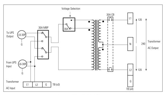
Figure 7. 9PXPPDM2 Block Diagram
