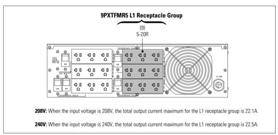
Figure 23. 9PXTFMR5 L1 Load Output Limits
