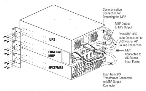
Figure 32. 9PXTFMR5, 11k 240V EBM, and 11k MBP with 9PX8000 or 9PX11000 UPS (Kits 9PX8KTF5 and 9PX11KTF5)
