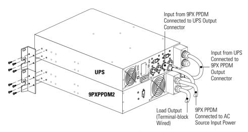
Figure 31. 9PXPPDM2 with 9PX5000 or 9PX6000 UPS (Kits 9PX5KP2 and 9PX6KP2)
